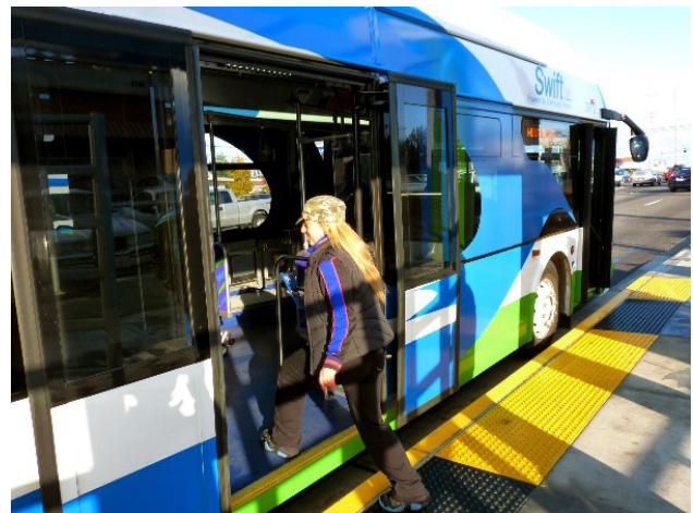
Multiple door boarding, as used on Community Transit's Swift BRT service, improves boarding/alighting speed
