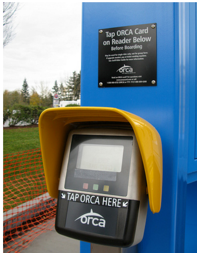
Ticket Vending Machines (top) and Smart Card Technology with Validators (bottom) are used for “Proof-of-Payment” fare collection
