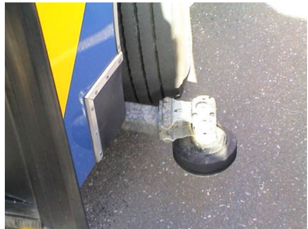
Mechanical docking system guides BRT vehicles for precise in-line boarding.
