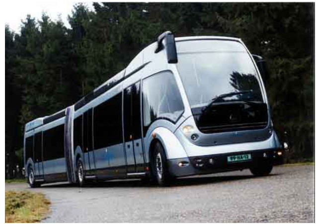
Multiple doors, articulation, and unique styling on the Phileas BRT vehicle
