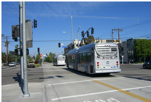
LA Metro's Orange Line operates on an at-grade, exclusive right-of-way
