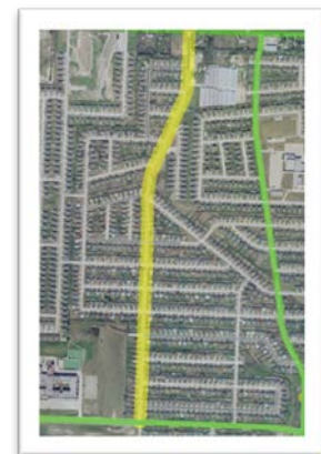
Figure 3-3: Example of Urban Minor Arterial
